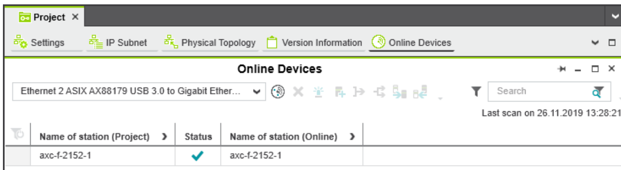
Figure 6-7 Successful assignment of the configured controller to an online device
